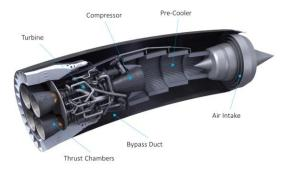
Figure 2: SABRE 3 (Reaction Engines)
